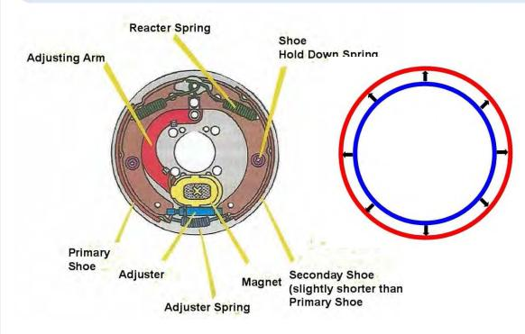
As the drum heats up, it will expand outward away from the brake shoes.
