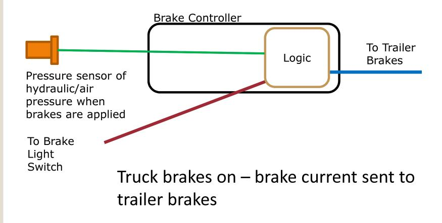
Hayes Air Actuated electric brake controller.
