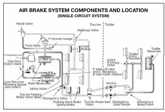
The Emergency air hose fills the Trailer reservoir. For brake actuators that have Parking springs, the Emergency air also releases the Parking springs.
