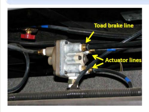
Dual Actuator Installation to gain enough fluid volume.
