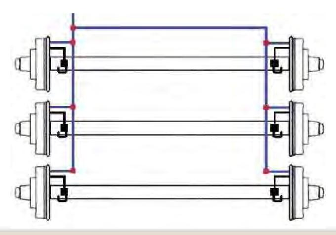
Better wiring for electric drum brakes
