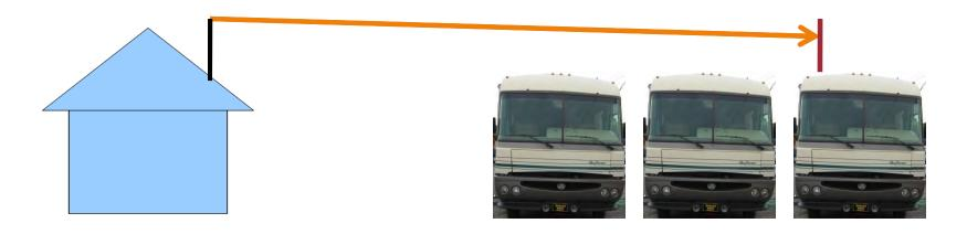
Roof mounted antenna will clear other RVs and have a direct shot at Park antennas.
