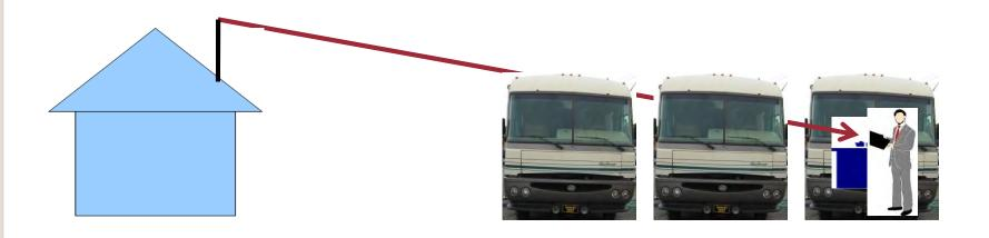
Roof mounted antenna will clear other RVs and have a direct shot at Park Wi-Fi
