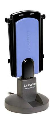
The USB wireless adapters are really integrated wireless radios and antennas. The USB cable has a length limit of 5 meters.
