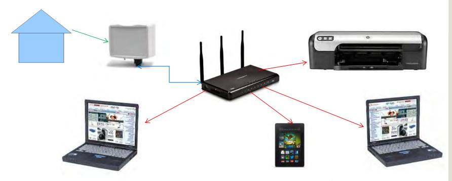
By using a CPE (Customer Premises Equipment) radio to connect to the Park Wi-Fi and connecting your wireless router to the radio, your PCs and Printer can communicate on you local LAN and to the Internet via the CPE.
