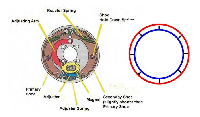
As the drum heats up, it will expand outward away from the brake shoes.
