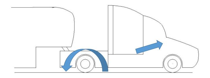
Typical HDT pin location: after the axle During braking, causes a rotation to the rear of the pin weight reducing the effective truck motion.
