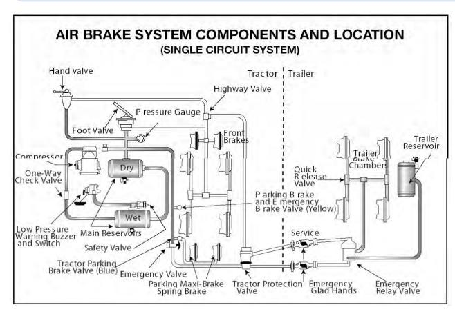
The Emergency air hose fills the Trailer reservoir. For brake actuators that have Parking springs, the Emergency air also releases the Parking springs.
