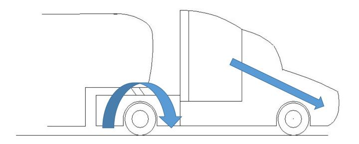
Typical pickup pin location: over axle During braking, causes a forward rotation of the pin weight amplifying the motion of the truck
