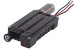
Air from the brake line causes a piston to push a rheostat to adjust the amount of current to the trailer brakes.
