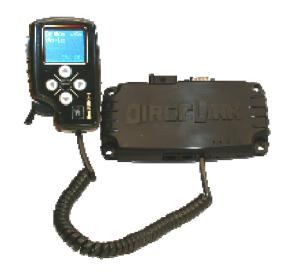
Tuson DirecLink was designed to connect to the OBD-II data ports of standard pickups.
