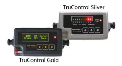
Hensley: Uses an inertia sensor like a small gyroscope that is not dependent on tilt for speed change detection.
