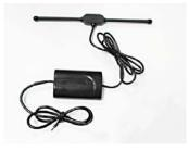
A second option is a signal repeater located between the monitor and the farther sensors (Toad)
